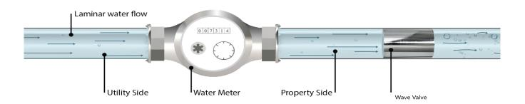
The AquaFlow Valve acts as a small restrictor with a minimum reduction of 5%. The system reduces from a certain diameter to a smaller diameter, running for just 3mm before opening to a full port (95%). On the other side (proprietary), there is no significant effect on flow or pressure. This process is very similar to the Venturi effect.
